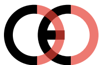
False CE Mark (too close)
